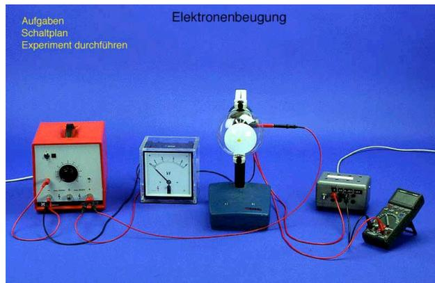
Figure 2: An interactive screen experiment for electron diffraction
