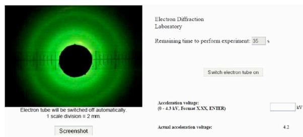
Figure 1: The approximate screen for the Kaiserslautern remote control electron diffraction experiment. (As they say on the airplane, it has been modified slightly to fit on the page.) <http://rcl.physik.uni-kl.de/>
